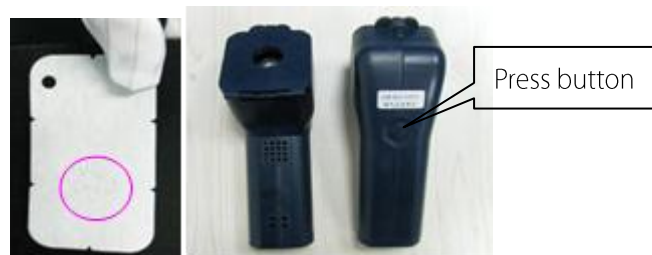
Fig.5-13Suction sampling paper (left) and Vacuum Sampling unit (right)
