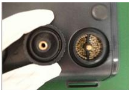
Fig. 6-6 Discarding the filled material
